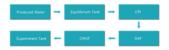
The oil contained wastewater firstly passes through the CPI unit to remove slick oil; then in the DAF unit emulsified oil will be largely reduced; finally
